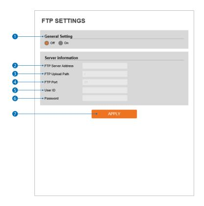
To send and save images from the camera to an FTPserver, an FTP needs to be setup.
