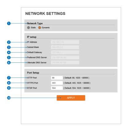
1 Network type - Set the camera's network type. Select Dynamic or Static IP.
