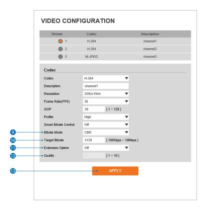
9 Bitrate mode - Select the bit rate control scheme of video compression from CBR (Constant Bit Rate) or VBR (Variable Bit Rate).
