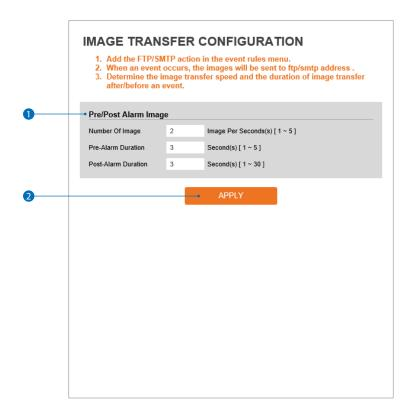
1 Pre- / post- alarm image - Image transfer due to event is configured by setting up the image transfer rate and pre and post alarm duration.
