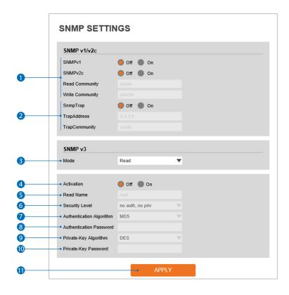
**1** SNMPv1/SNMPv2 - Select the SNMPv1/SNMPv2 option and type the names of read community and write community.
